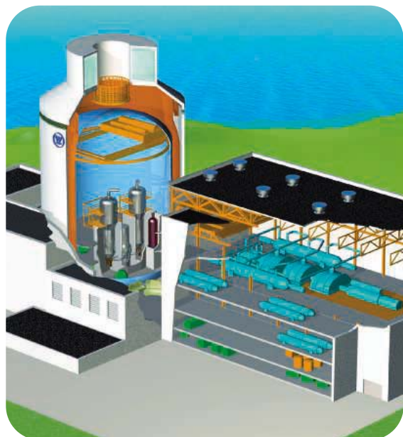
Gentle giant. Westinghouse's AP1000 design now has passive safety systems using gravity and natural circulation.
